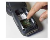
Insert the microSD card with the written part upward. Lock the card into place by pushing the cardholder down and then sliding it to the left.
