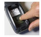
5. Replace the battery (see Battery Installation).
