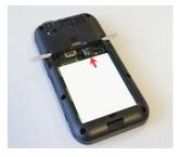
4. Replace the battery (see **Battery Installation**).
