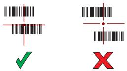
Figure 4-7 Pick List Mode with Multiple Bar Codes in Aiming Pattern
