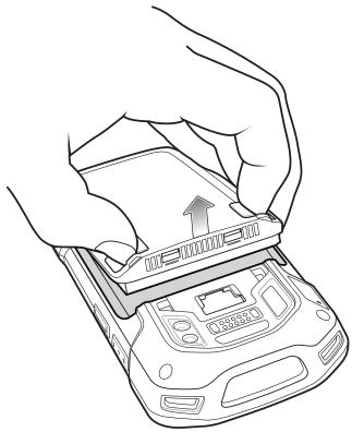
Figure 1-13 Lift the Battery
