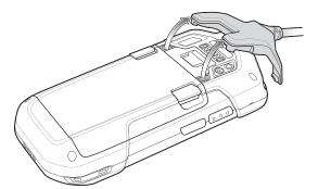
Figure 6-45 Remove Cable from TC70
