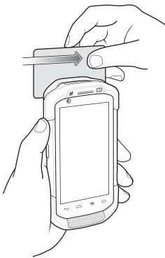
Figure 6-20 Swiping a Magnetic Stripe Card
