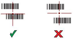
Figure 4-4 Pick List Mode with Multiple Bar Codes in Aiming Pattern
