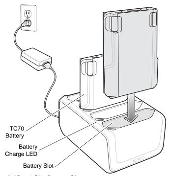
Figure 6-15 4-Slot Battery Charger
