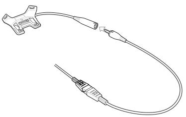
Figure 6-29 Connect Adapter Cable to Audio Adapter
