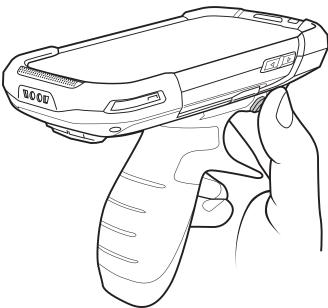
Figure 6-51 Press Release Latches
