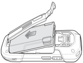
Figure 1-6 Insert Bottom of Battery into Battery Compartment
