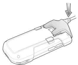
Figure 6-44 Press Down on Cable
