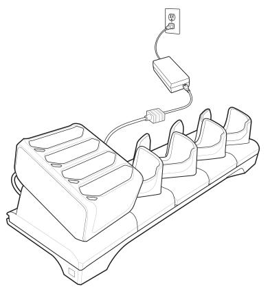
Figure 6-11 5-Slot Charge Only Cradle with Four Slot Battery Charger
