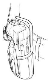
Figure 6-25 Device with Audio Adapter in Holster
