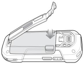
Figure 1-7 Press Down on Battery
