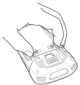
Figure 1-12 Press Battery Latches
