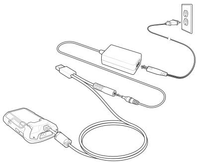
Figure 6-35 Power Setup
