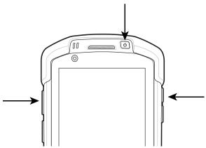
Figure 2-14 Three Button Reset
