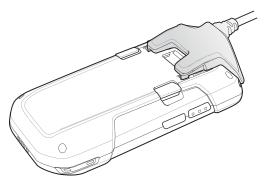
Figure 6-42 Cable Attached to TC70
