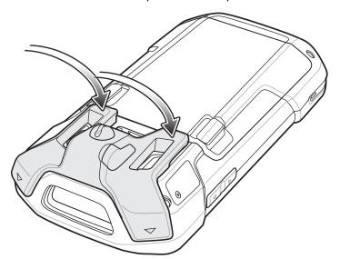
Figure 6-22 Rotate Audio Adapter onto TC70
