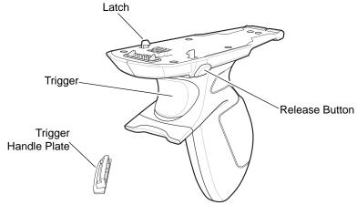
Figure 6-46 Trigger Handle
