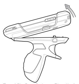
Figure 6-52 Rotate Device onto Trigger Handle
