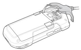
Figure 6-37 Remove Cable from TC70
