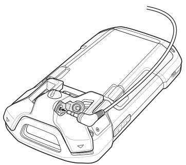
Figure 6-23 Connect Headset to Audio Adapter
