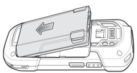
Figure 1-9 Insert Bottom of Battery into Battery Compartment
