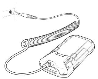
Figure 6-43 DEX Cable Connection
