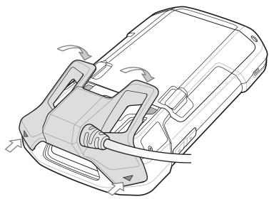
Figure 6-27 Audio Adapter Installation
