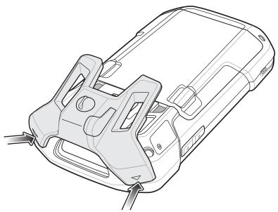
Figure 6-21 Audio Adapter Installation
