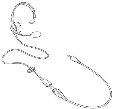
Figure 6-28 Connect Headset to Adapter Cable
