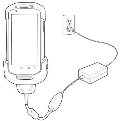
Figure 6-40 Connect Cable to Power Supply
