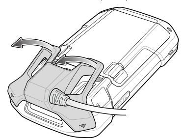
Figure 6-31 Remove Audio Adapter from TC70
